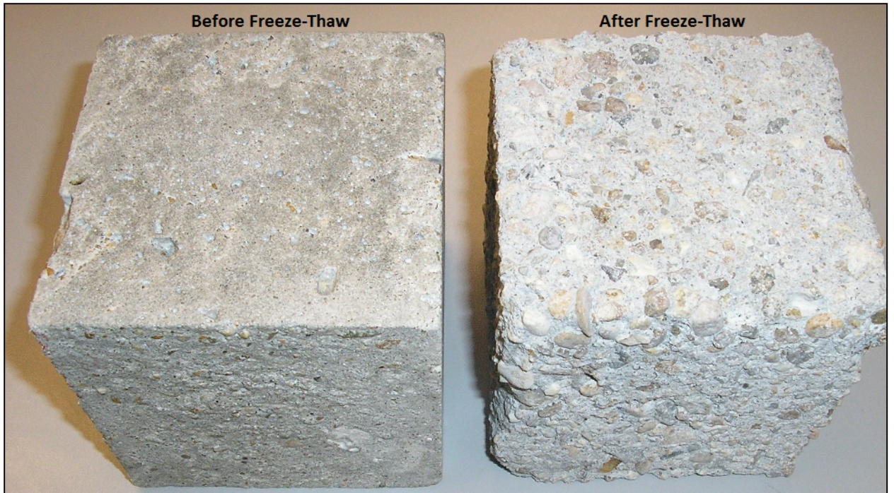
Figure 5.2 Silane Before and After 300 Freeze-Thaw Cycles
